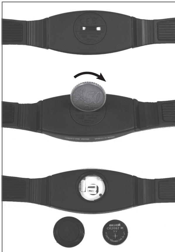
OPENING THE BATTERY COMPARTMENT OF THE CHEST STRAP
