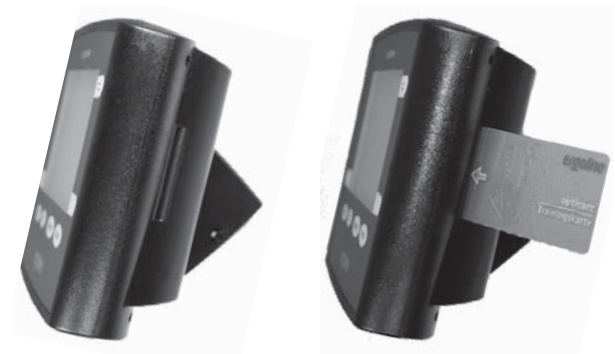
CHIP CARD READER IN THE OPTIBIKE
